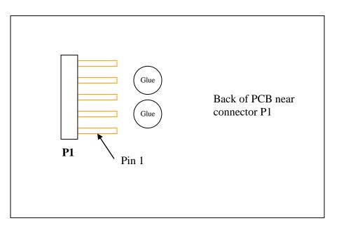
Add a dab or two of glue on the PCB just in front of the connector so that the cable header will sit on the glue when connected to the board and make itself more secure. The picture above illustrates the placement of the glue prior to the connection
